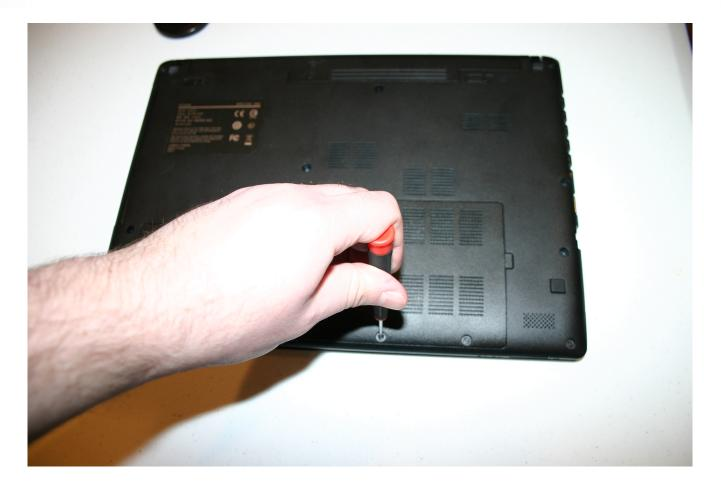
2. Pull up on the tab shown in red to remove the cover (slowly and carefully).
