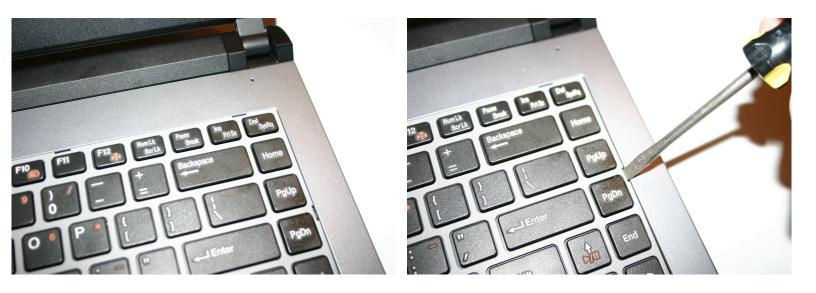
Using a flat head screw driver insert into the latch holes on keyboard. Press down to eject keyboard.
