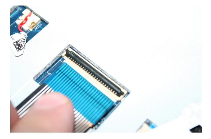
A picture before insertion of the keyboard's cable.
