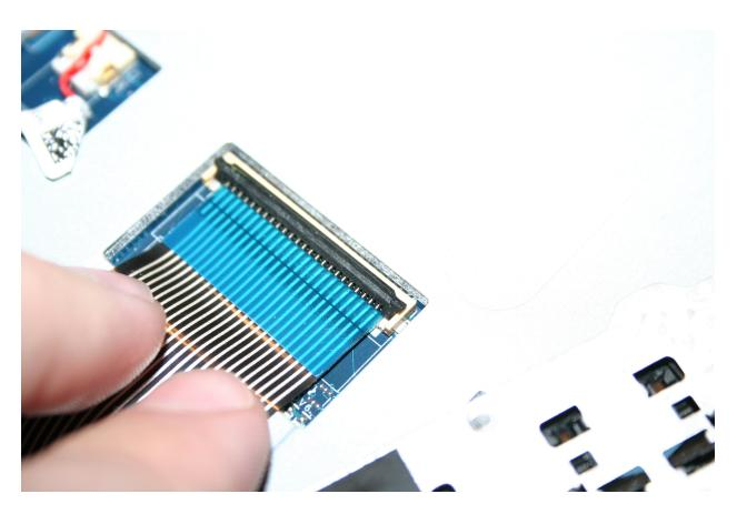
A picture after insertion of the keyboard's cable.
