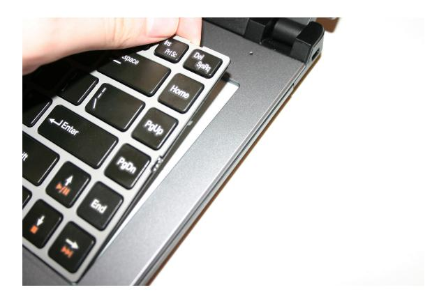
Lift keyboard. Use flat head screw driver to get "up" if needed. Be careful not to use force here.
